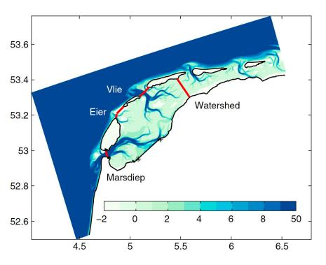
Wind effect on transport of suspended sediment (model results):
