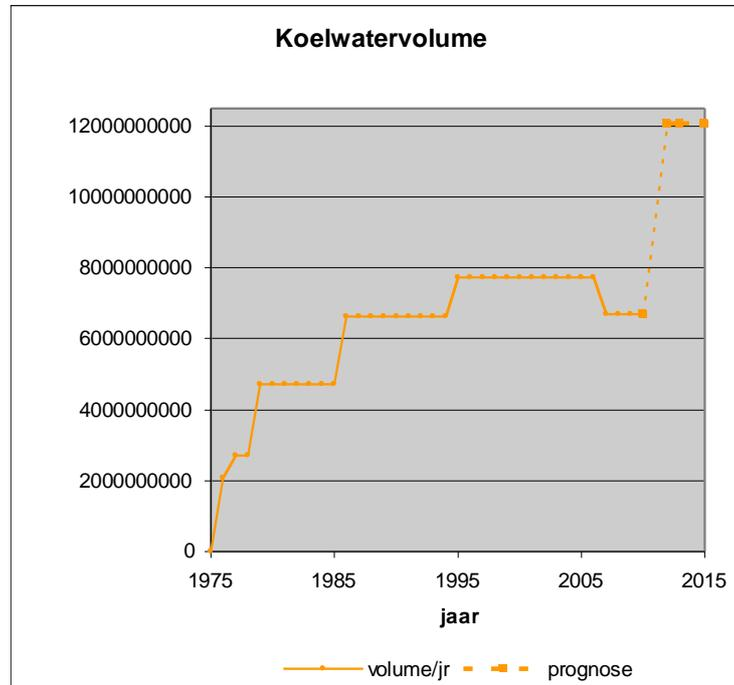
Figure 2. Trends in annual cooling water volume (m<sup>3</sup>) by power plant >500 MW along the Wadden Sea coast and estuaries in the Netherlands, Germany and Denmark, calculated from data in Table 2.
