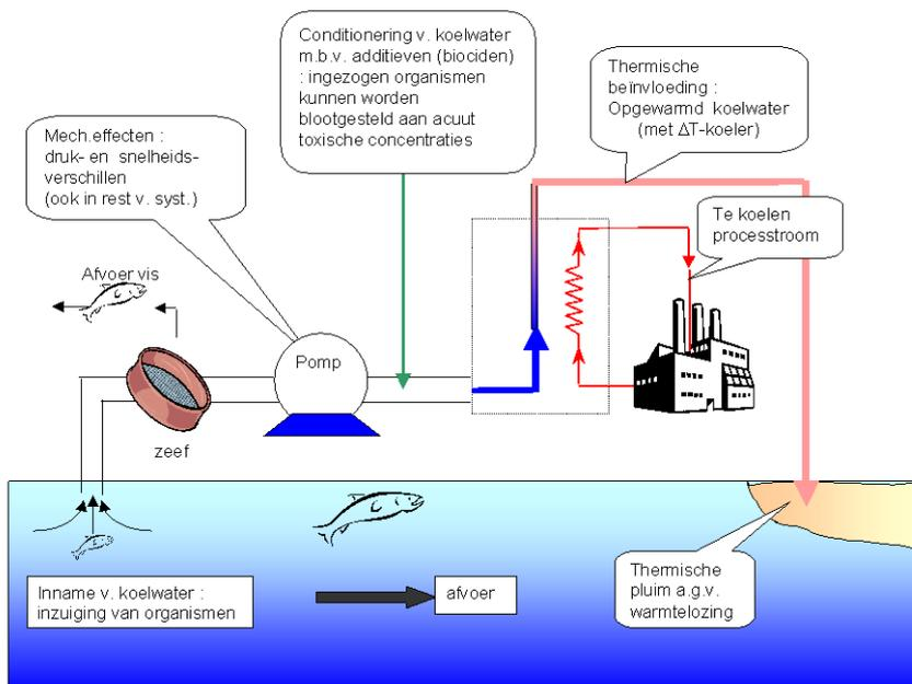
Figure 1. Schematic representation of cooling water used in electricity generation (CIW, 2005).
